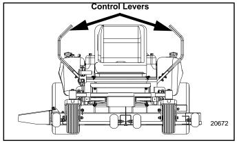
Control Levers in Parking Brake Position Figure 2-5
